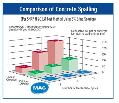
3% test concentrations of brine were used since ice melter brine typically dilutes itself to this level soon after it is applied. After 15 freeze/thaw cycles, the use of sodium chloride resulted in over 63 times and calcium chloride resulted in over 26 times the amount of concrete loss than MAG.
