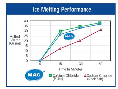
The tests were performed by the Swedish VTI by spreading 10 grams of each ice melter evenly over an icy surface at  $21^{\circ}F$ , well within the performance range of sodium chloride. As the temperature drops, the performance of sodium chloride should degrade appreciably as it reaches its practical minimum melting point of  $+6^{\circ}F$ .
