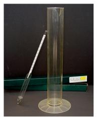
and higher as density of the material increases. Understanding that water is specific gravity of 1.00, we want the hydrometer to settle in this solution at 1.322 to tell us that is on specification.
